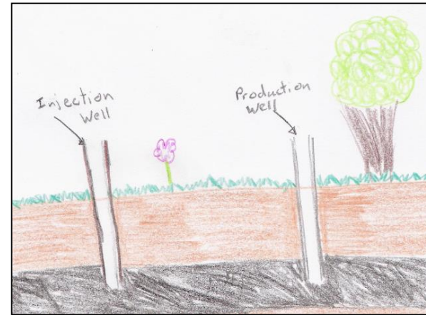
Drill the boreholes
