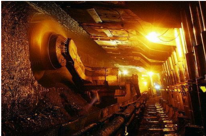
Large Mining-Height Longwall Face
