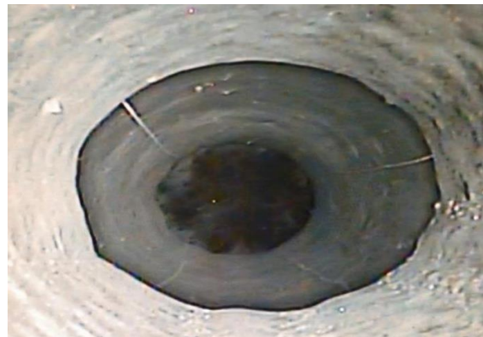
气化炉内壁中段挂渣情况 Slag coverage around center of the liner
