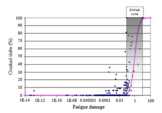
Figure 3. Fatigue damage-slab cracking model used in the MEPDG.
