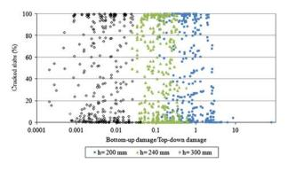
Figure 1. Predicted JPCP slab cracking as a function of the ratio of bottom-up damage to top-down damage for various slab thicknesses.
