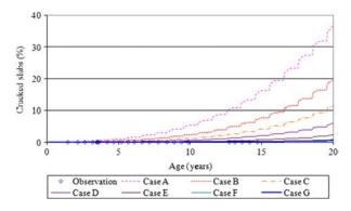
Figure 2. Prediction of slab cracking of Cell 13 for various PCC property inputs.
