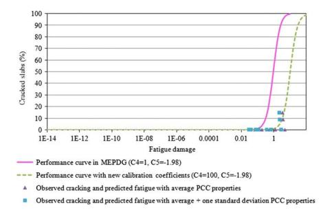
Figure 4. MEPDG performance curve vs. locally calibrated performance curve.
