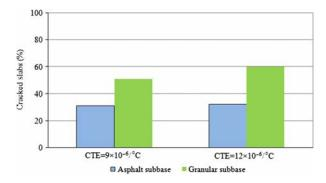
Figure 7. Effects of subbase type on JPCP slab cracking for different CTEs.
