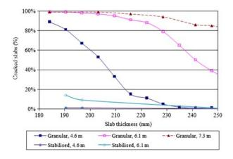
Figure 5. Sensitivity of predicted JPCP slab cracking to slab thickness, subbase type and joint spacing.
