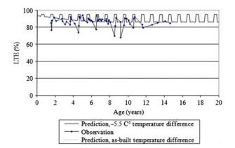
Figure 8. Predicted and observed LTE for Cell 11.
