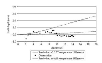
Figure 10. Predicted and observed faulting for Cell 6.
