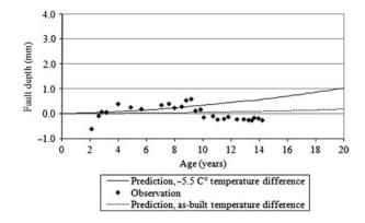
Figure 9. Predicted and observed faulting for Cell 11.
