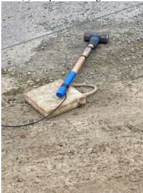
(c) Sledge hammer and board used to generate signal
