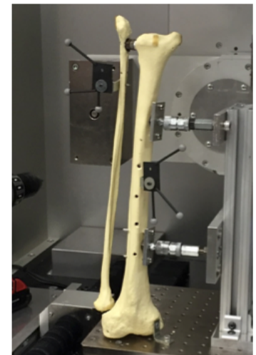
Figure 4. Experimental setup for translational accuracy test. Both triads can be seen from all camera orientations.
