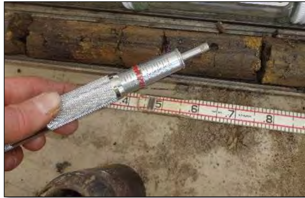
Figure 7-1 - Field Hand Penetrometer Reading
