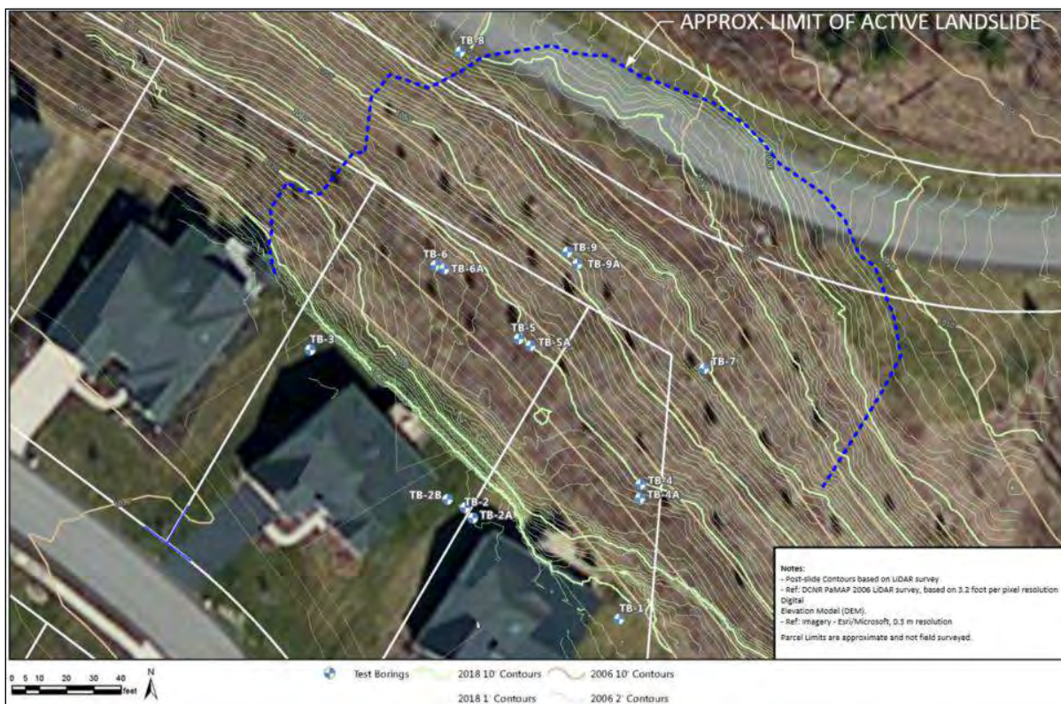
Figure 4-7 - Sample boring plan including offset borings for undisturbed sample collected as well as subsequent inclinometer and piezometers installations
