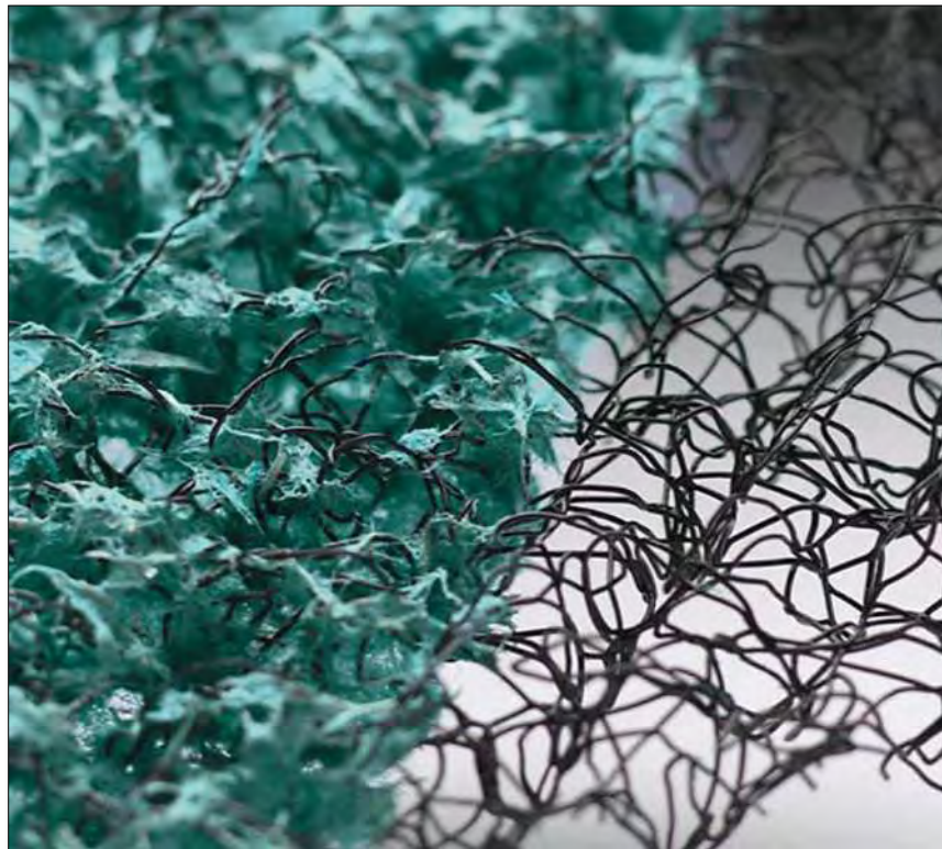
Figure 10-26 - Green Armor TRM System with Flexterra Flexible Growth Medium
