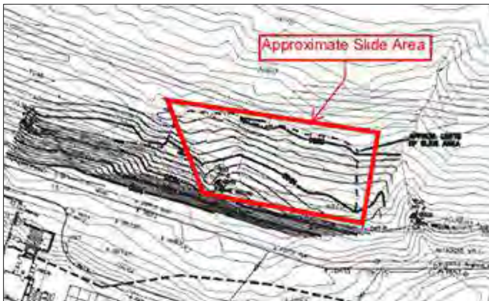
Figure 4-2 - Cut slope constructed within a topographically anomalous area resulted in a slope failure
