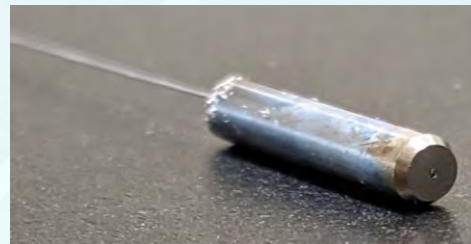
Aluminum-coated optical fiber soldered into a stainless-steel ferrule. This is the first step in fabricating a variety of fiber-optic-based sensors.
