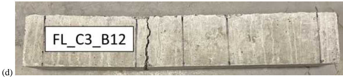
(d) Figure 52: Failure cracks for (a) FL_C5_B5 (age = 4-day) (b) FL_C4_B1 (age = 3-day) (c) FL_C6_B8 (age = 17-day) (d) FL_C3_B12 (age = 20-day).
