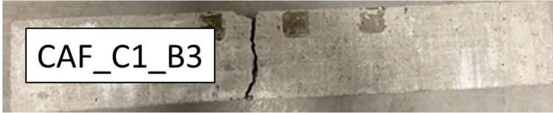
Figure 57: Failure cracks for (a) CAF_C3_B3 (age = 4-day) (b) CAF_C4_B4 (age = 4-day) (c) CAF_C2_B9 (age = 22-day) (d) CAF_C1_B3 (age = 27-day).
